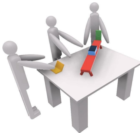
Figure 3. 3D-sketch showing students' positions while they measure the speed of the car. While discussing the results, all the students are behind the computer C (yellow). The measuring apparatus, A, consisting of the track (red), the car (blue) and the ultrasound sensor (green).
